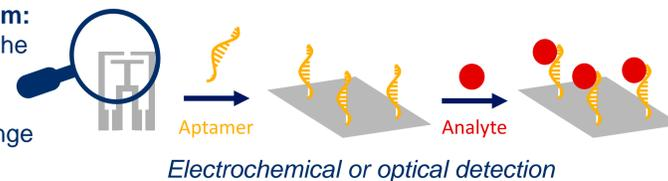
**Pros/Cons:** aptamers are cheaper and more stable than antibodies. Standard functionalization protocols available. Sensitive to unspecific binding
