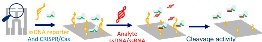
**Biosensing mechanism:** CRISPR/Cas enzyme activated by gRNA sequence acquire unspecific cleavage activity in presence of the gRNA complementary strand. ssDNA cutting on sensor cause a detectable change.
