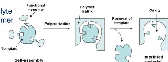
**Pros/Cons:** no need of a bioreceptor and theoretically stable over time but the polymer-template mixture and the polymerization conditions are long and difficult to optimize. Typically low reproducibility.
